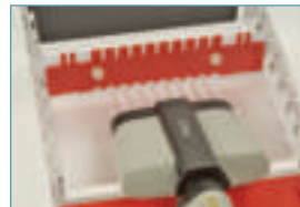
combi-comb/guides offer the convenience of a regular comb with a loading guide (same teeth number and width), simply by flipping over
